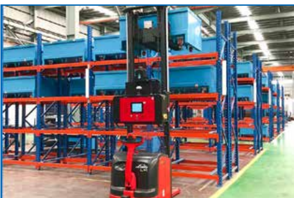
Forklift AGV system detects itself by Laser
