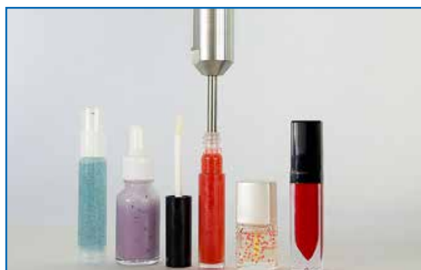
The system can extract materials with a hardness of up to 7,000,000cps / mPas
