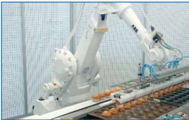
The robot automatically picks up the cake into the tray
