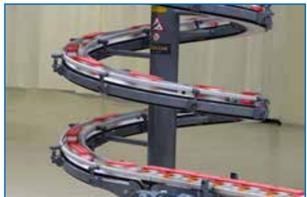
Spiral Elevator conveyor system brings products up to save space
