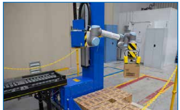
The UR10 with Zero stand design can be folded in 2 pallets
