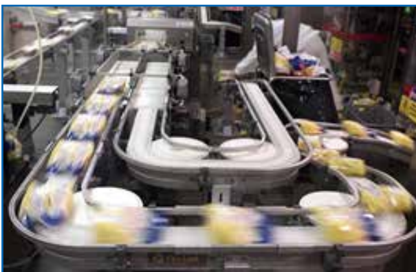
High-speed conveyor in the food industry with U-shaped and S-shaped curves
