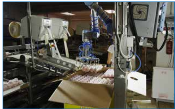
Universal Robot application automatically crates eggs
