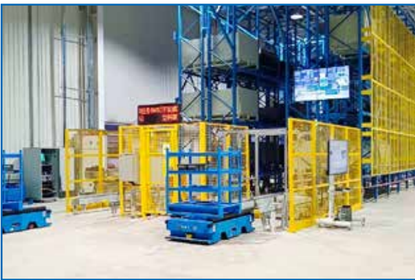
Truck AGV system leads the way with magnetic tape
