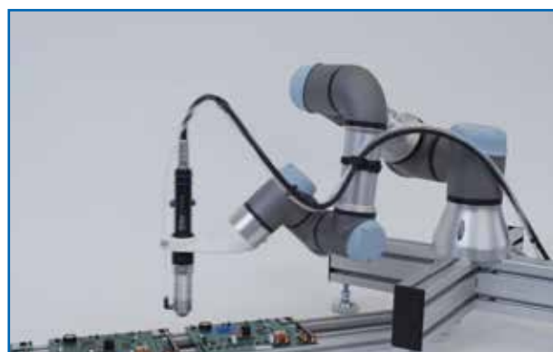
Application Universal robot and ViscoTec Spray spray protection circuit board
