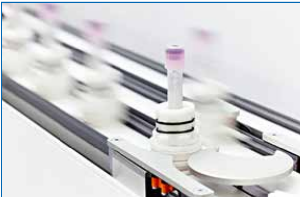
Puck conveyor system used in Pharmaceutical - Chemical industry
