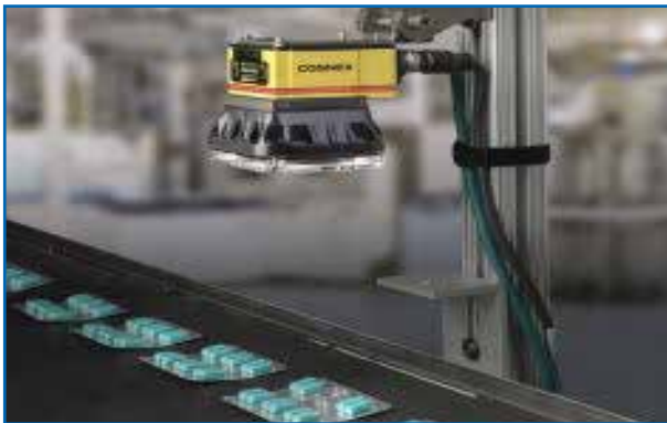
Automatic capsule inspection system
